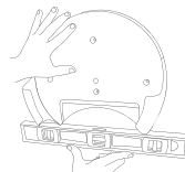
Figure 1: Use a level when placing wall mount against surface
